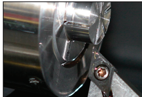
Detail of burr causing problems for a manufacturer of medical heart pumps.
